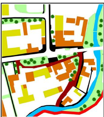
Figure 1: Possible re-alignment of junction to enhance parking and safety also provide on street car parking
